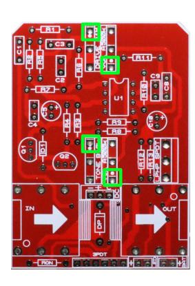
Then, solder them to the board like in the picture in the left, and then place the board inside the enclosure:
