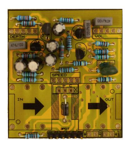
Solder the capacitors and transistors. If you have troubles reading the values, check out our <u>"Reading Part Values"</u> tutorial. Pay attention to the orientation, as well as to the polarity for electrolytic capacitors.
