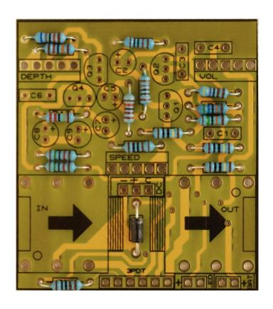
Place the resistors and diodes. If you have troubles reading the values, check out our <u>"Reading Part Values"</u> tutorial.
